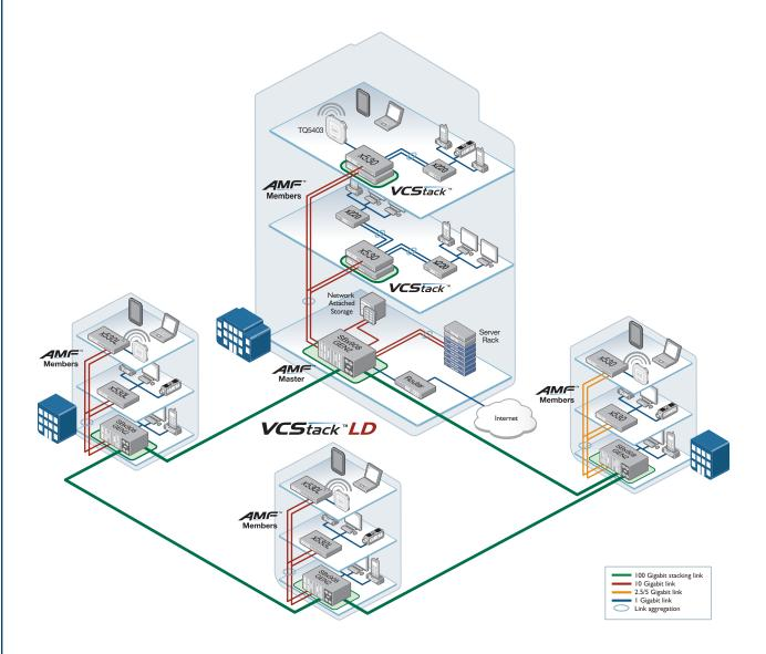
Today's large enterprises demand ready access to online resources and applications, and require a high-performing network that can seamlessly carry multiple converged services. This campus solution uses the SwitchBlade x908 GEN2 and VCStack LD—ideal for a distributed network core that provides high availability, increased capacity and ease of management.
