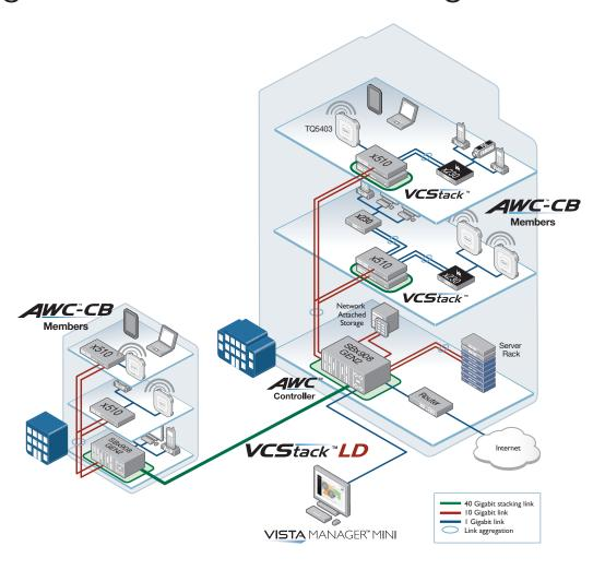
Allied Telesis Autonomous Wave Control (AWC) offers solutions for two of the most common problems with Wireless LANs: initial setup complexity, and on-going performance degradation. Initial WLAN set-up usually requires a site survey to achieve the best coverage, and performance of WLANs can often change over time as external sources of radio interference reduce coverage and bandwidth. These issues can be time-consuming to identify and resolve.
